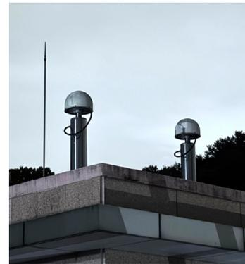
Fig. 4. GPS antennas in static experiment.
