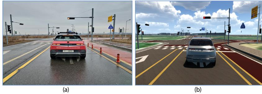
Fig. 3. Digital Twin in K-CITY: (a) a real vehicle in real environment, and (b) a virtual vehicle in driving simulator with digital twin of (a).
