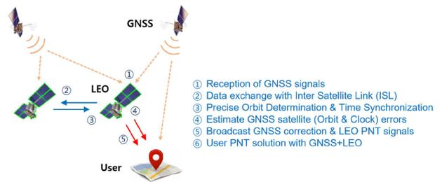
Fig. 10. Proposed LEO PNT utilization scenario.
